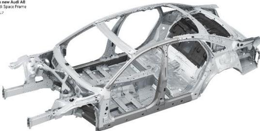
An intelligent combination of four different materials will be used for the first time in the body structure of the next generation Audi A8. This also affects the company's future automation strategy.
