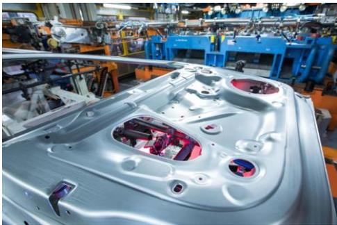
Audi is optimizing quality control at the pressing plant using artificial intelligence.
