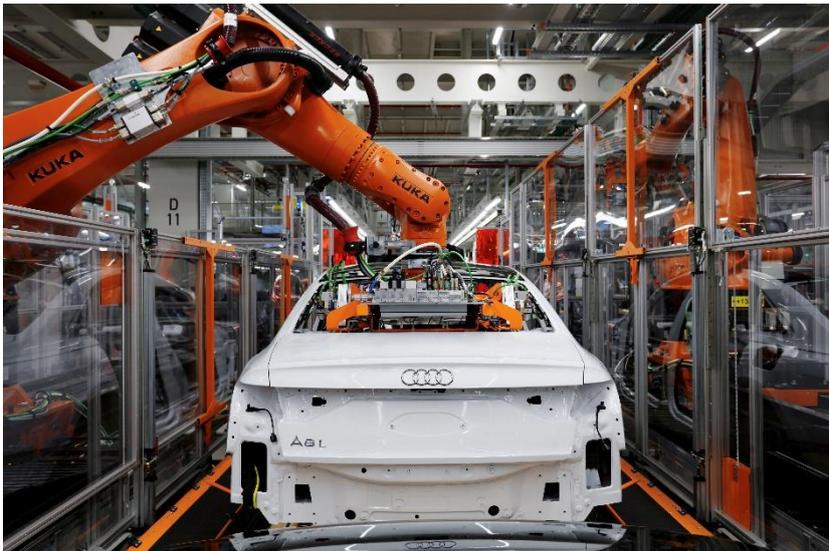
Audi A8: Installation of the CFRP rear wall at the Neckarsulm site
