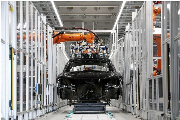
Audi A8: Installation of the panorama glass roof at the Neckarsulm site
